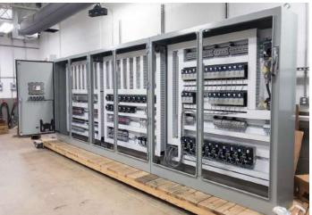
LV Control panel is a component of an electrical control system that regulates and monitors low voltage circuits. It is used in a variety of applications such as HVAC, water treatment plants, manufacturing, and industrial automation.
